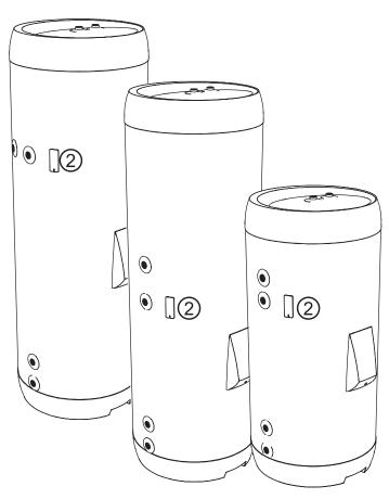
The temperature sensor (1) can be fitted in the electric junction box as shown below, or in the factory fitted EPP sensor pocket (2). The EPP sensor pocket accepts both 6 and 8 mm. sensors.
