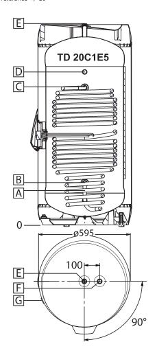
Coil is filled when installing external heat source. Follow instructions supplied with external heat source or contact approved installer.
